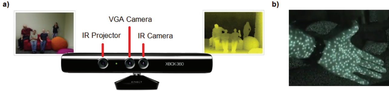
Fig. 1 - a) Microsoft Kinect schematic; b) Kinect's Infra-Red projection pattern.
